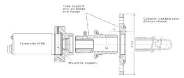
Schematic drawing of the flange system
