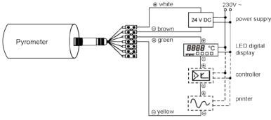
Connection Schematic for Analyzing Devices
